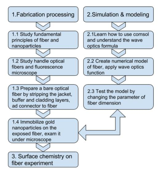
The flowchart shown above is showing the stages of the experiment for the first semester. We will start with fabrication processing of optical fiber, at the same time, we will learn how to use simulation software to create numerical simulation to select the best parameter of optical fiber. After we finished handling the optical
